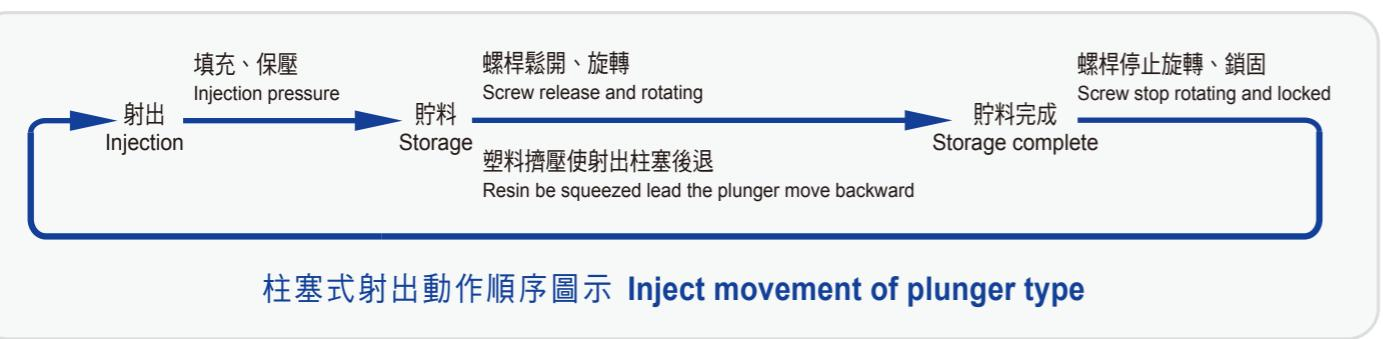
柱塞式射出動作順序圖示 Inject movement of plunger type
